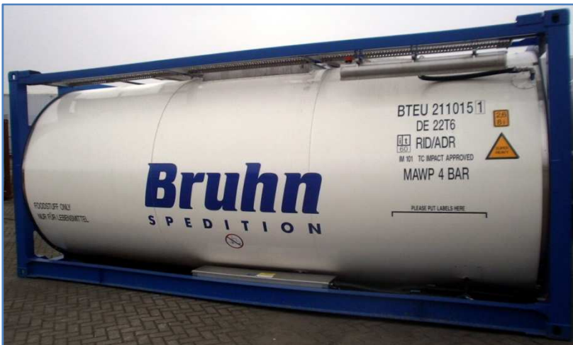
Tank-Container with special insulation and GRP lagging
