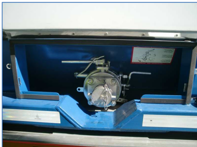
Fully enclosed discharge area with DN 80 Fort Vale floor valve and 3" BSP thread
